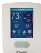
The Daikin *Adaptive Touch Controller* (ATC) is used to control FDMQ and FFQ (P1P2) indoor units with advanced and configurable control logic. The ATC comes in 4 different models with a built-in temperature sensor, humidity sensor, CO<sub>2</sub> sensor, and occupancy sensor. The
